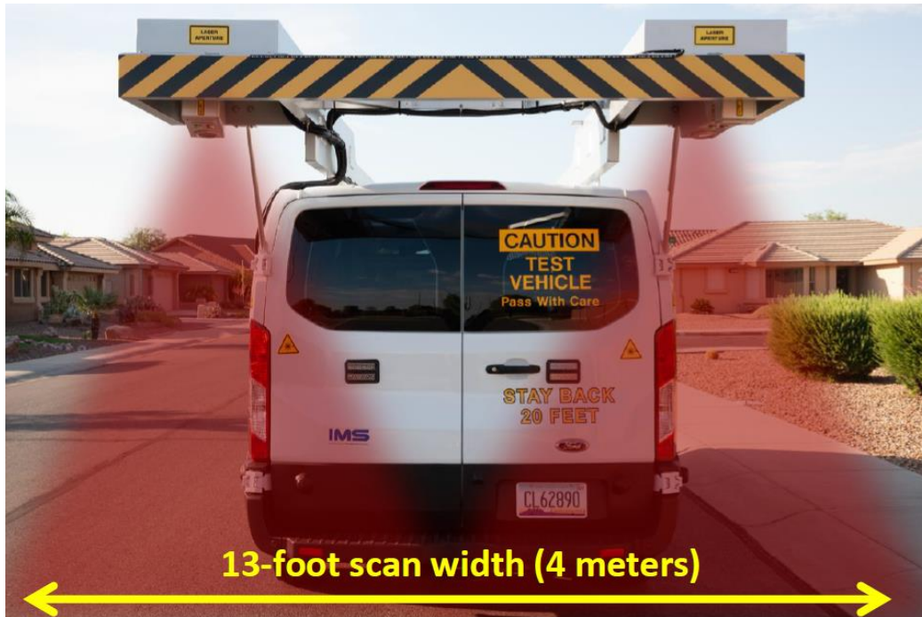
Figure 5 – RST Equipped with the 3D LCMS-2 Camera
