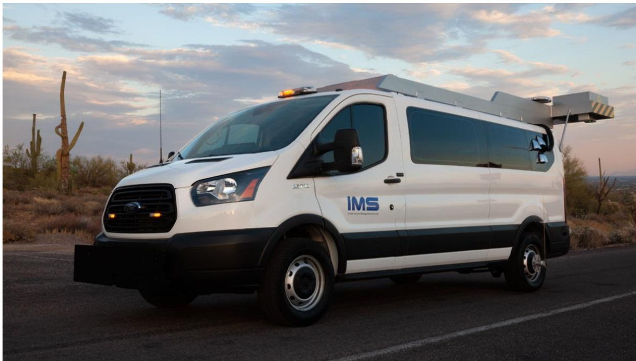
Figure 4 - Laser Road Surface Tester (RST)
